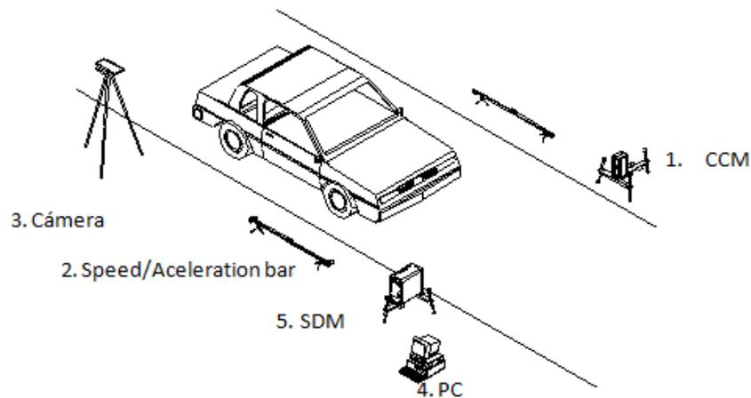
Figure 2-1 Basic scheme of Opus RSD components
