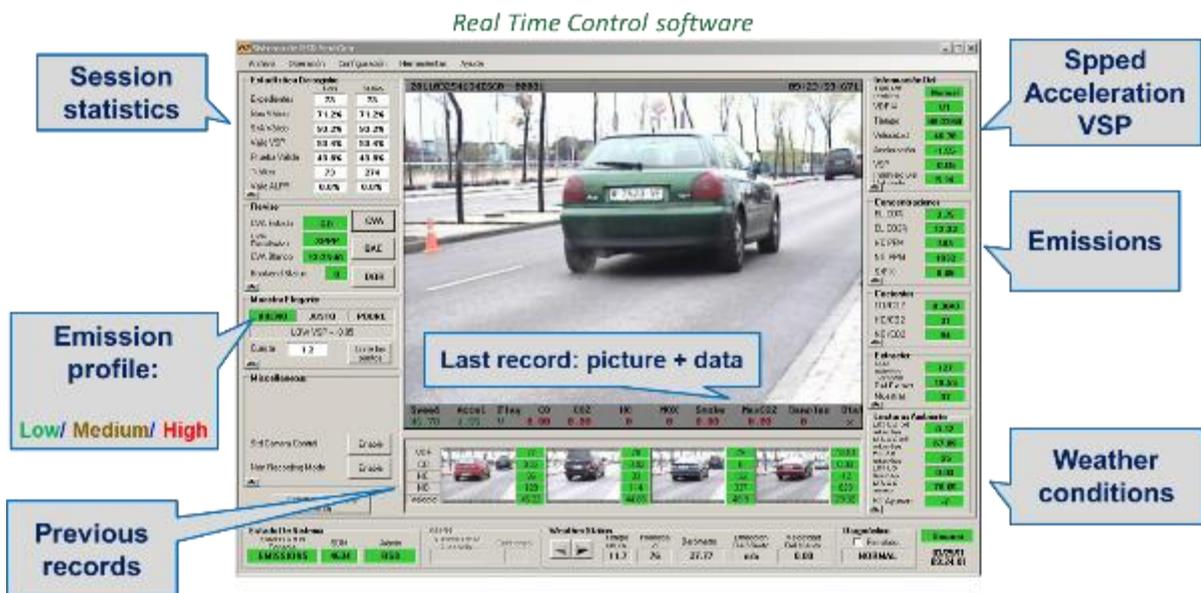
Figure 3-3 Sample of a vehicle measurement screen plot in Opus real-time monitoring software
