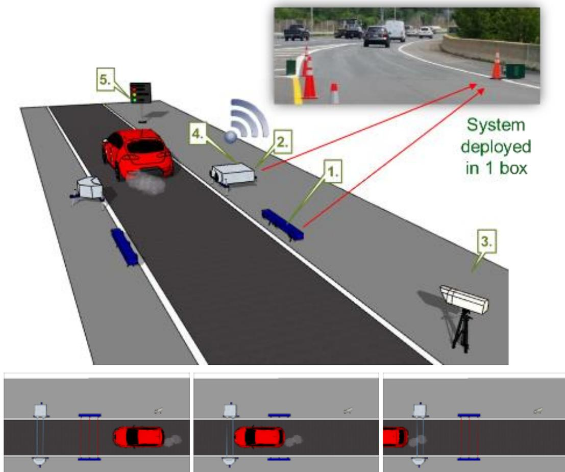
Figure 3-2 Scheme of a measurement with Opus RSD
