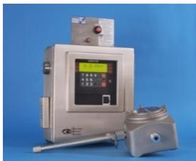
Acoustic monitor of particles in liquids, oil in water, water in oil and air bubbles
