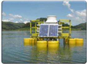
Reservoir profilers to determine contamination and algae content in different depth. The system is solar powered and a wrench is moving the analytic set up and down.
