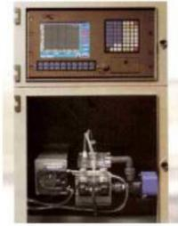
Heavy metal analyzers for online monitoring of trace levels of metallic pollutants in water. Multicomponent modules allow a compact design of monitoring stations.
