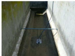
Portable and stationary flow monitoring instrumentation allows reliable monitoring of waste water flow in tubes or open channels.
