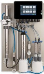
On-line monitoring of organic and inorganic water quality compounds Typically COD, TOC, DOC, NO<sub>3</sub>, TSS, NH<sub>4</sub>, EC, DO, pH are monitored and a spectral alarm system allows to generate an alarm in case of increased concentration of contaminants such as pesticides, aromatic hydrocarbons, nerve-paralytic agents or others.
