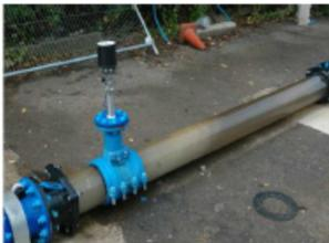
In-situ monitoring of contaminants allows to be installed directly in the pressurized water pipes with no need to stop operation and measuring the important disinfection or contamination parameters.
