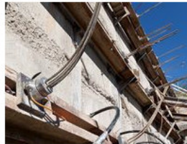
Load cell PRE 1000/100/80 monitoring a retaining wall
