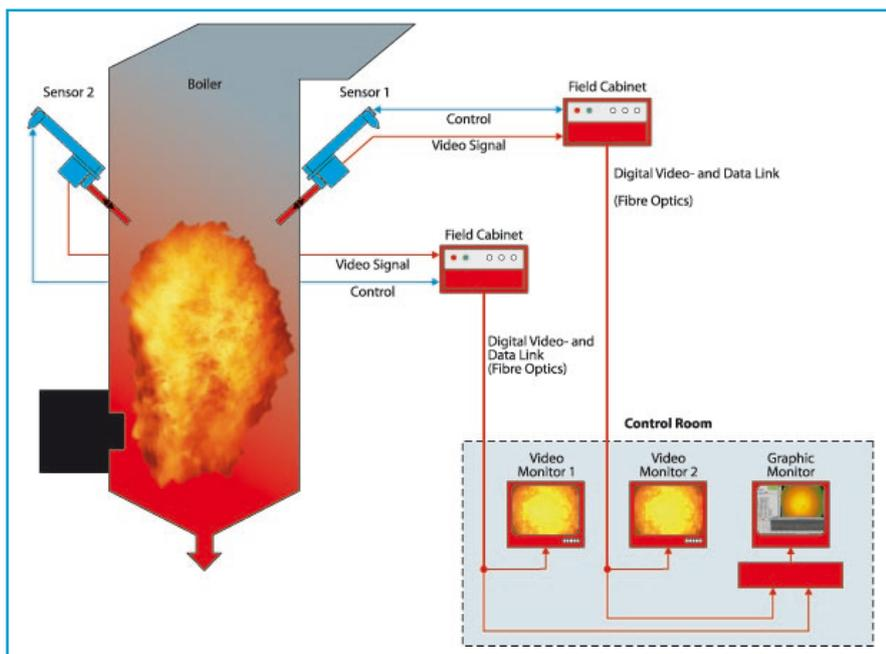
Figure 1: Diagram illustrating DURAG's Video and Thermography System monitoring combustion in the furnace.
